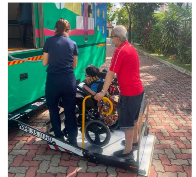
A Mobile Dental Clinic with a special lift to transfer patients on wheelchairs into the clinic.
